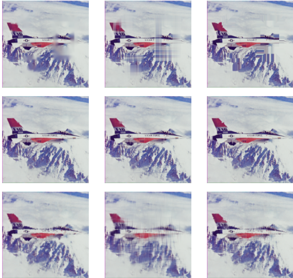
Figure 98: Reconstruction of the image avion . The rows are from top to bottom for masks holes , scratches , noise from Fig. 2. The technique used for reconstruction is the same for column, where the first is the F-transform, the second is the bilinear interpolation and the third is the nearest neighbor.
