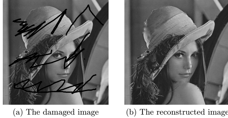
Figure 40: The damage caused by scratches from Fig.2c or manual painting removed by one-step F-transform.
