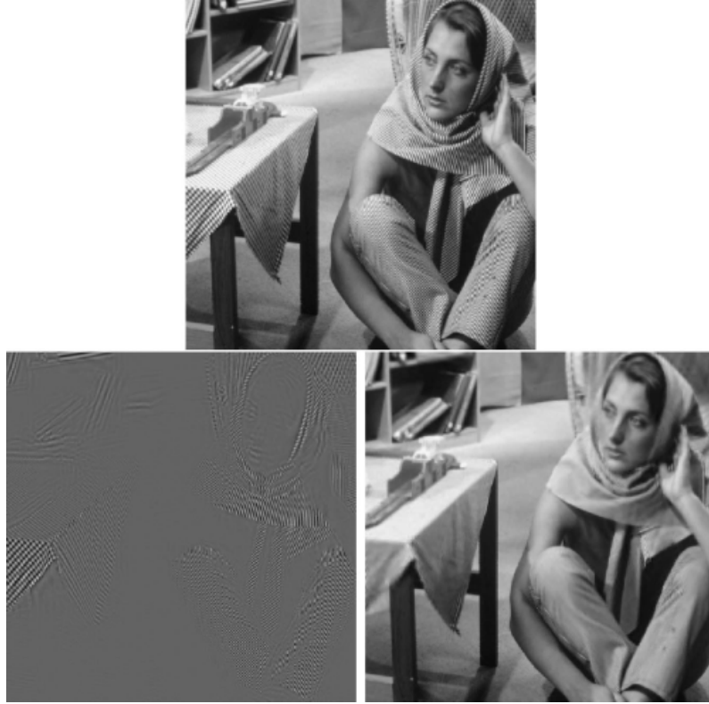
Figure 30: Separated texture (bottom left) and geometry (bottom right) from photography by Elad et al. (figure taken from [11])
