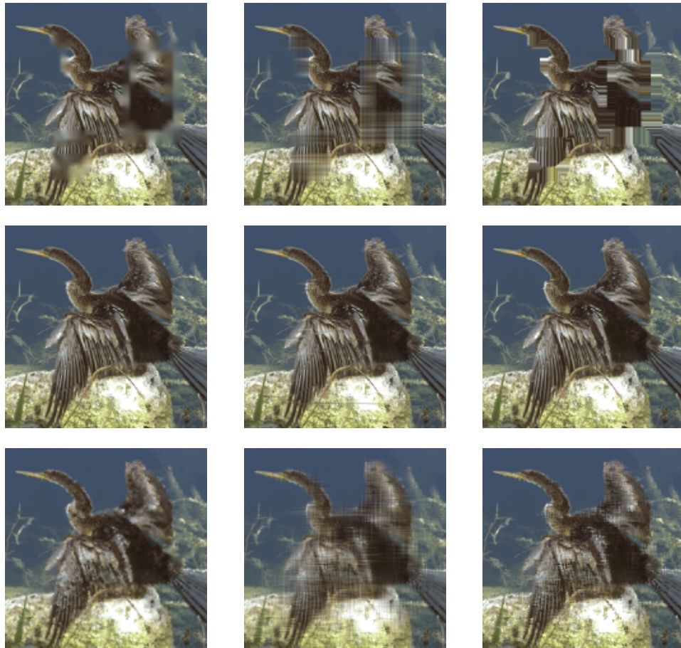
Figure 95: Reconstruction of the image anhinga . The rows are from top to bottom for masks holes , scratches , noise from Fig. 2. The technique used for reconstruction is the same for column, where the first is the F-transform, the second is the bilinear interpolation and the third is the nearest neighbor.
