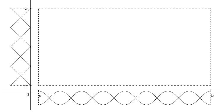
Figure 3.2: Uniform fuzzy partition of \mathcal{D}^2 comprised from sinusoidal and triangular shaped basic functions.
