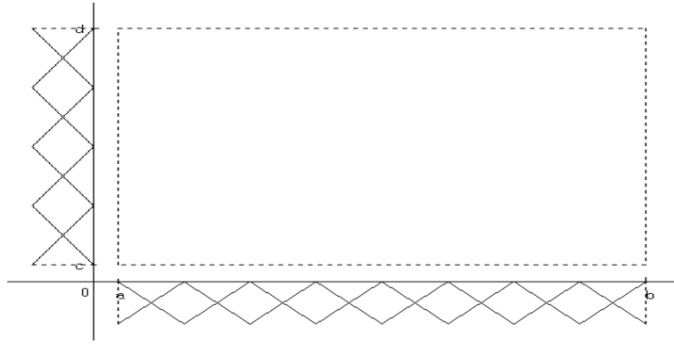
Figure 3.1: Uniform fuzzy partition of \mathcal{D}^2 comprised from triangular shaped basic functions on both axes.
